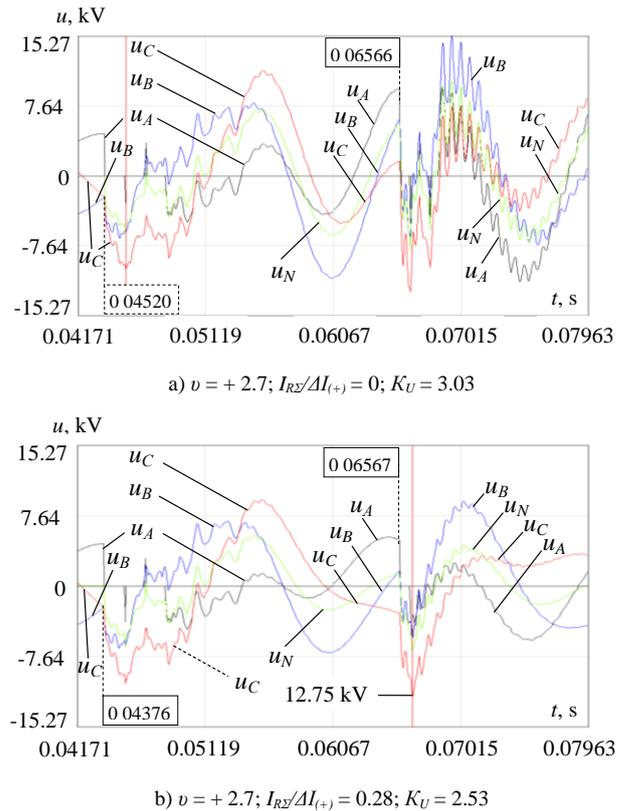
Fig. 2. Transient process at arcing ground fault at the beginning of a feeding cable at the 1st Busbars Group of the 6 kV main switchgear at CHP Plant with a compensation (a) and with a combined neutral grounding,  $R_{N\Sigma} = 100$  Ohm (b)
