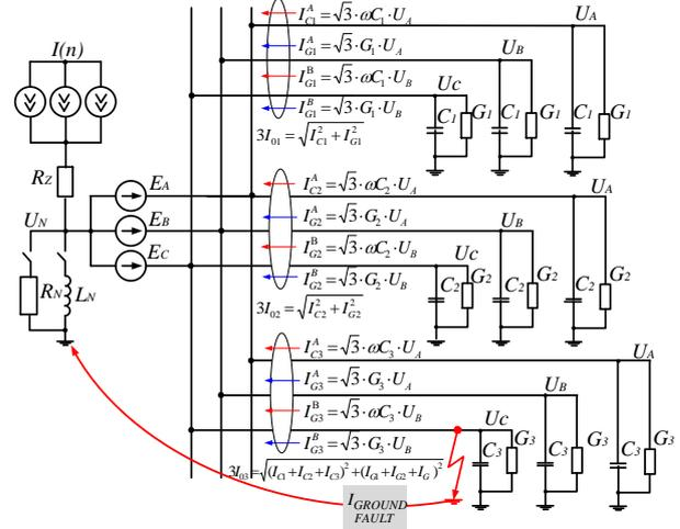
Fig. 1. Simulation model of a combined grounded network for the analysis of transient processes at single phase-to-ground faults with higher harmonic distortion currents (the model is applicable for the 1st Busbars Group and the 2nd Busbars Group, separately)
