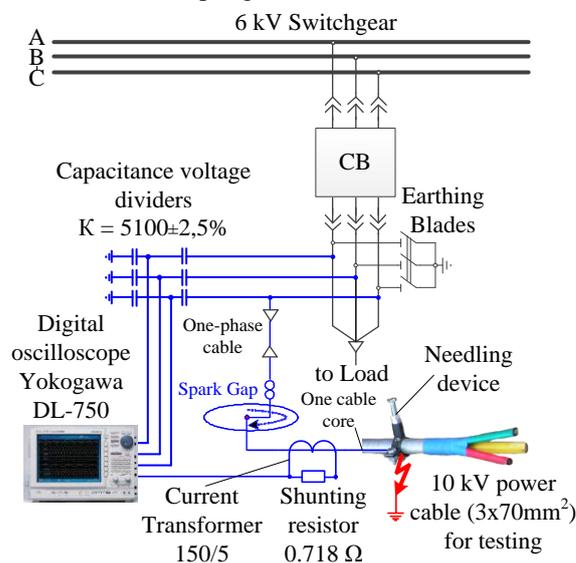
Fig. 1. The experimental circuit for the 6 kV network with arcing ground faults in the MIPI cable
