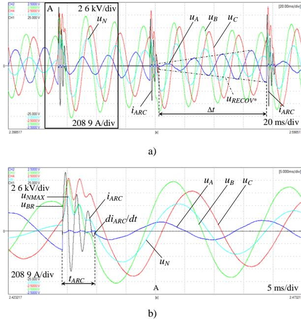
Fig. 2. Real oscillogram (a) and its fragment (b) of serial single-phase breakdowns in the MIPI cable insulation during experiment.
