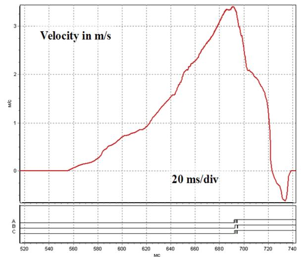
Fig. 6. The change of contact closure velocity for VMP-10-20/630 oil circuit breaker
