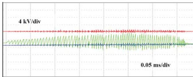
Fig. 7. Oscillograms of transient processes for phase-to-ground voltages at the moment of contact rebound at closing of VVTE-M-10-20/630 vacuum circuit breaker made by ENEKO Minusinsk
