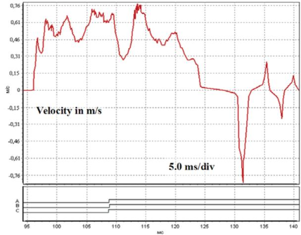
Fig. 4. The change of contact closure velocity for VBP-10-20/630 vacuum circuit breaker made by Kontakt Saratov
