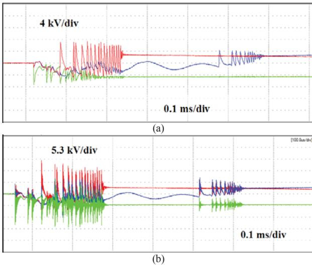
Fig. 1. Oscillograms of transient processes for phase-to-ground voltages at the beginning (a) and at the end (b) of the cable line at closing of BB/TEL-10-20/1000 vacuum circuit breaker made by Tavrida Electric Moscow in the 6 kV network
