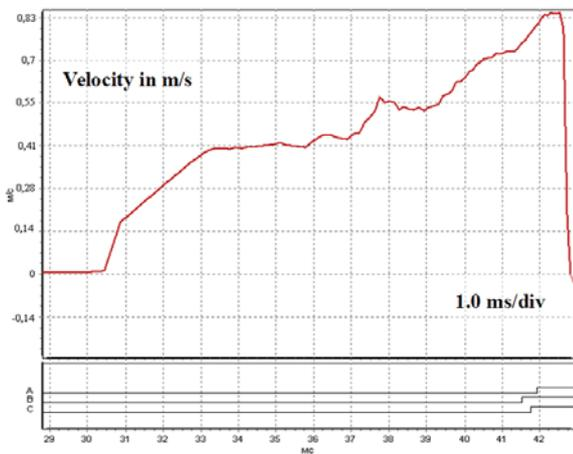
Fig. 3. The change of contact closure velocity for BB/TEL-10-20/1000 vacuum circuit breaker made by Tavrida Electric Moscow
