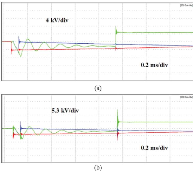
Fig. 2. Oscillograms of transient processes for phase-to-ground voltages at the beginning (a) and at the end (b) of the cable line at closing of VMP-10-20/600 oil circuit breaker
