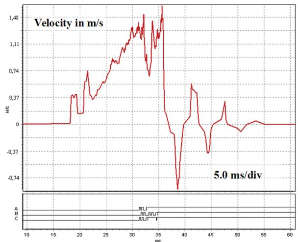
Fig. 5. The change of contact closure velocity for VVTE-M-10-20/630 vacuum circuit breaker made by ENEKO Minusinsk
