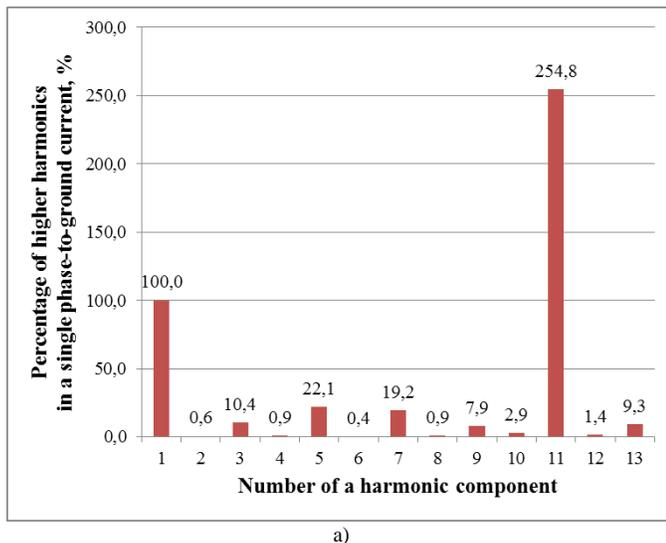
Fig. 2. Histograms of relative harmonic composition of single phase-to-ground current (a) and phase-to-ground voltage (b) in the 6 kV network of the urban CHP plant
