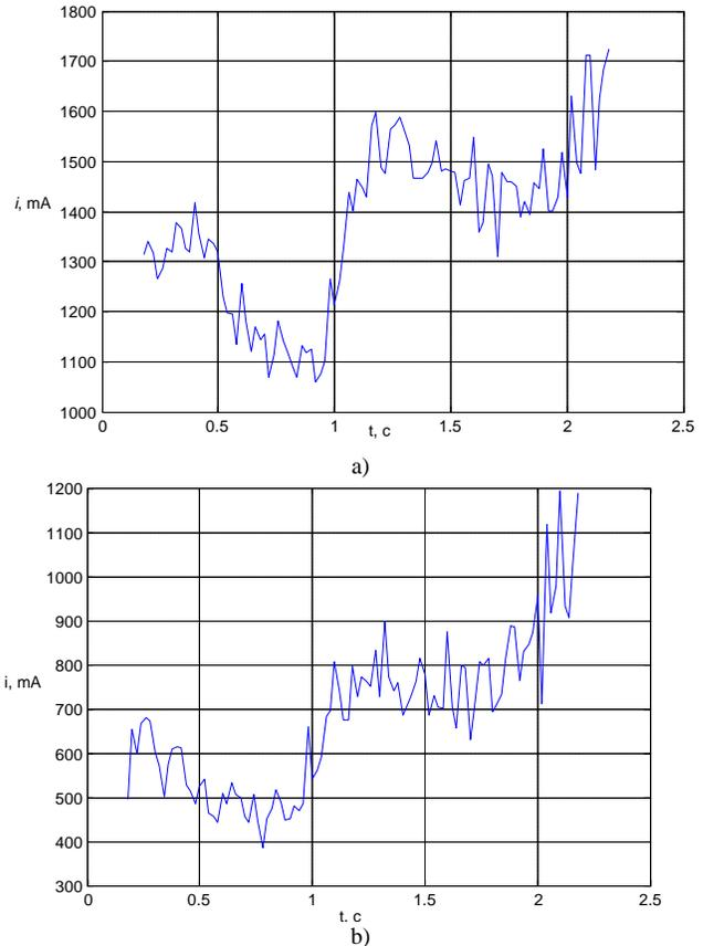
Fig. 3. Time changed process for the 35th (a) and 37th (b) harmonic amplitudes of single phase-to-ground current in the 10 kV network equipped with various ore-thermal furnaces
