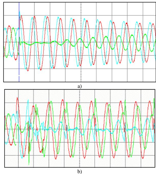
Fig. 4. Oscillograms of phase-to-ground voltages at single phase-to-ground arcing faults in the 6 kV resonant grounded network:
