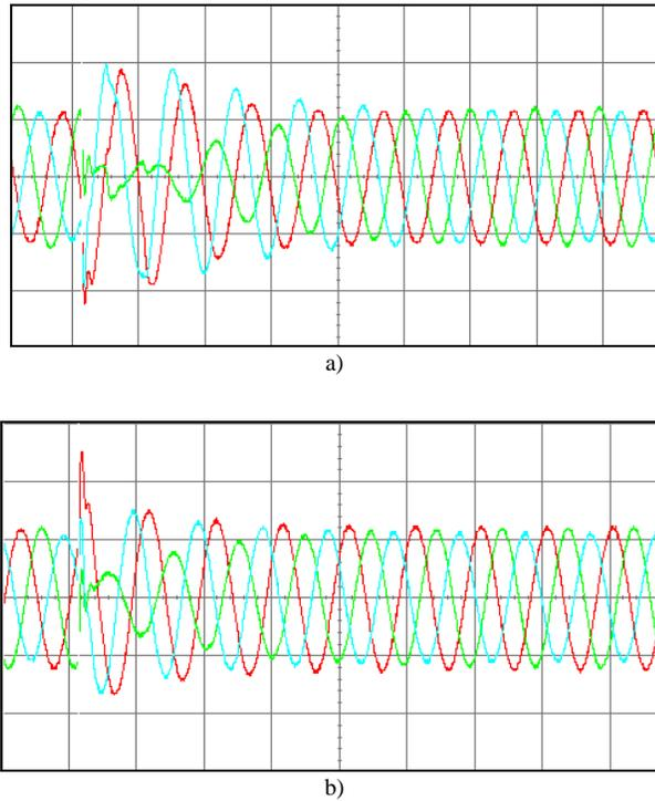
Fig. 5. Oscillograms of phase-to-ground voltages at single phase-to-ground arcing faults in the 6 kV combined grounded network:
