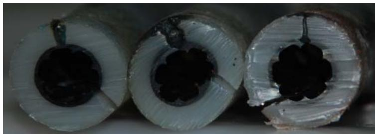
Fig. 4. Electric breakdowns of insulation in radial direction for 10 kV XLPE cables with short-time (up to 1 min) application of 50 Hz test voltage of 35–50 kV
