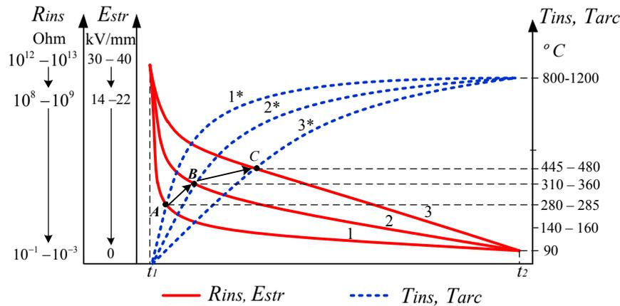
Fig. 3. Development of insulation breakdown for XLPE and EPR cables with time ( $R_{ins}$  – insulation resistance,  $E_{str}$  – electric strength,  $T_{ins}$  – insulation temperature,  $T_{arc}$  – arc column temperature) depending on different rates of breakdown channel development and applied 50 Hz voltage.
