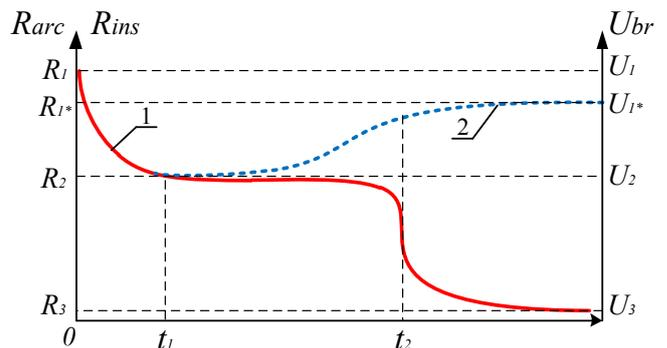
Fig. 1. Change of arc resistance (i.e. resistance of the arcing channel) and breakdown voltage for mass-impregnated paper-insulated cables during the development of arcing ground fault: 1 – development of non-cleared fault, 2 – breakdown channel pouring and self-recovery of insulation.
