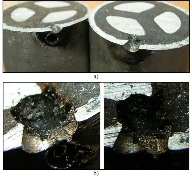
Fig. 2. Mismatch between a place of an artificial fault (i.e. an artificial insulation defect) and a place of real radial breakdown between a sector cable core and a grounded cable sheath (fig. a) and the result of arcing in a mass-impregnated paper-insulated cable (fig. b) during experiments and investigations on arcing ground faults in the operational 6 kV network.
