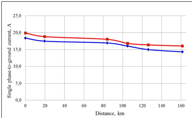
Fig. 2. Capacitance current distributions along the transmission line obtained from the model (red curve) and from investigations on operational power lines (blue curve)
