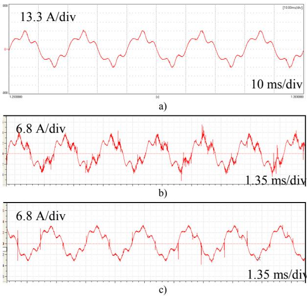
Fig. 10. Real oscillograms of single phase-to-ground currents recorded in various points of the transmission line: a) Sosnovka Substation; b) Satnur Substation; c) Kilmez Substation.
