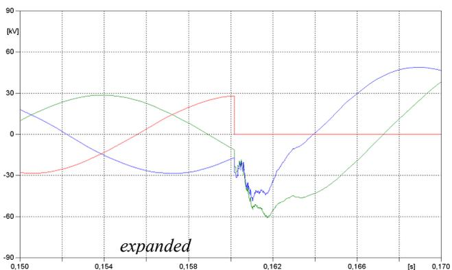
Fig. 7. Calculated oscillograms of phase-to-ground voltages recorded at Astrakhanovo Substation at single phase-to-ground fault at Astrakhanovo Substation.
