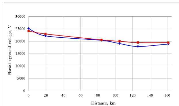
Fig. 1. Calculated (red curve) and recorded (blue curve) voltage distributions along the transmission line obtained from the model and from investigations on operational power lines.
