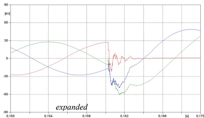
Fig. 8. Calculated oscillograms of phase-to-ground voltages recorded at Orlovskaya Substation at single phase-to-ground fault at Astrakhanovo Substation.
