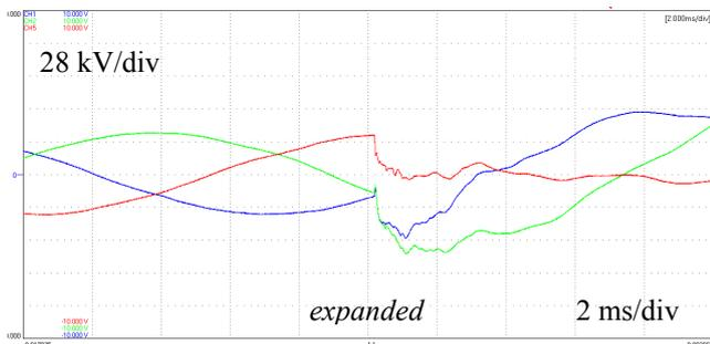
Fig. 3. Real oscillograms of phase-to-ground voltages recorded at Sosnovka Substation at single phase-to-ground fault at Astrakhanovo Substation.
