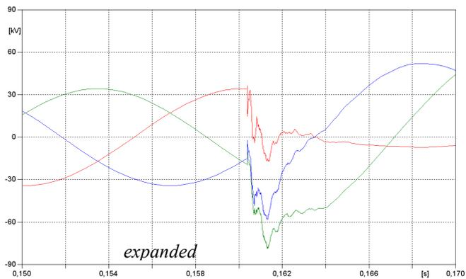
Fig. 6. Calculated oscillograms of phase-to-ground voltages recorded at Sosnovka Substation at single phase-to-ground fault at Astrakhanovo Substation.
