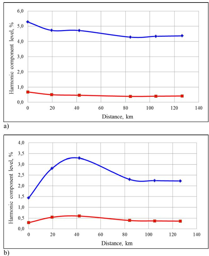
Fig. 12. Harmonic composition of calculated (red curve) and recorded during experiments (blue curve) single phase-to-ground current in various points of the transmission line: a – 250 Hz harmonic; b – 350 Hz harmonic
