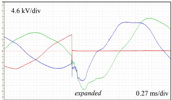
Fig. 4. Real oscillograms of phase-to-ground voltages recorded at Astrakhanovo Substation at single phase-to-ground fault at Astrakhanovo Substation.
