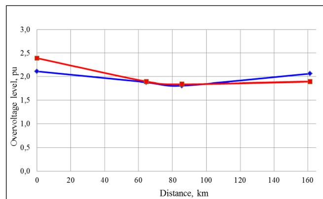
Fig. 9. Overvoltage levels along the transmission line at solid single phase-to-ground fault at Astrakhanovo Substation calculated from the model (red curve) and recorded during investigations on operational power lines (blue curve).
