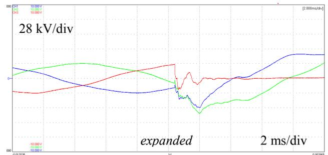
Fig. 5. Real oscillograms of phase-to-ground voltages recorded at Orlovskaya Substation at single phase-to-ground fault at Astrakhanovo Substation.
