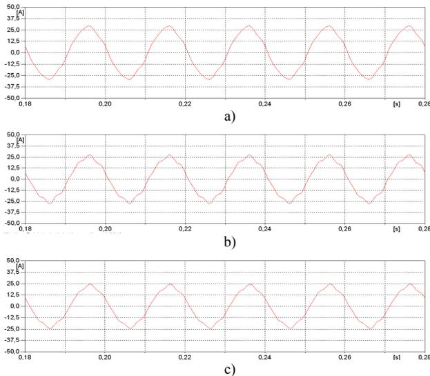
Fig. 11. Calculated oscillograms of single phase-to-ground currents in various points of the transmission line: a) Sosnovka Substation; b) Satnur Substation; c) Kilmez Substation.
