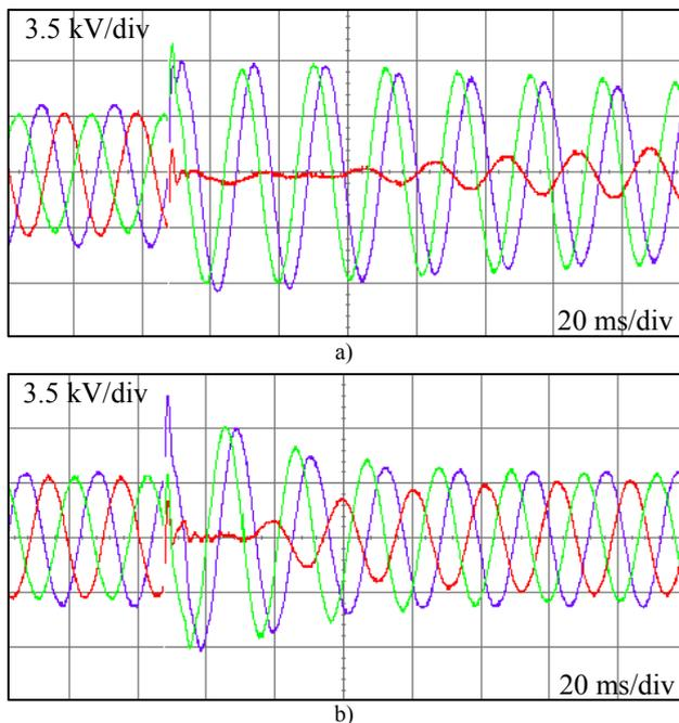
Fig. 2. Oscillograms of transient processes at single phase-to-ground faults in the 6 kV network of NKMK:
