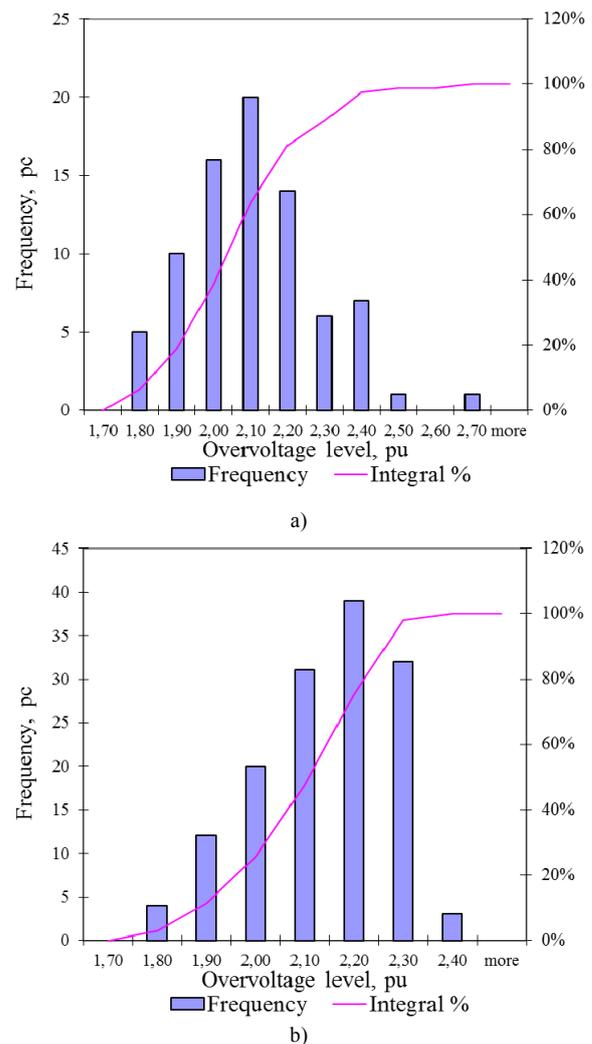
Fig. 3. Frequency distributions of overvoltage levels in the 6 kV network of NKMK (a – Petersen coil, b – Petersen coil + Resistor).
