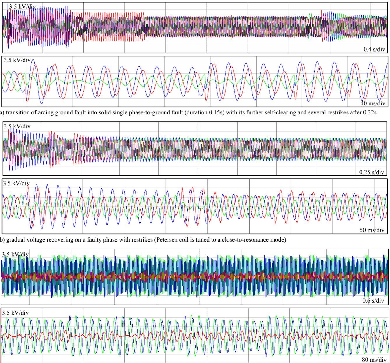
a) transition of arcing ground fault into solid single phase-to-ground fault (duration 0.15s) with its further self-clearing and several restrikes after 0.32s
