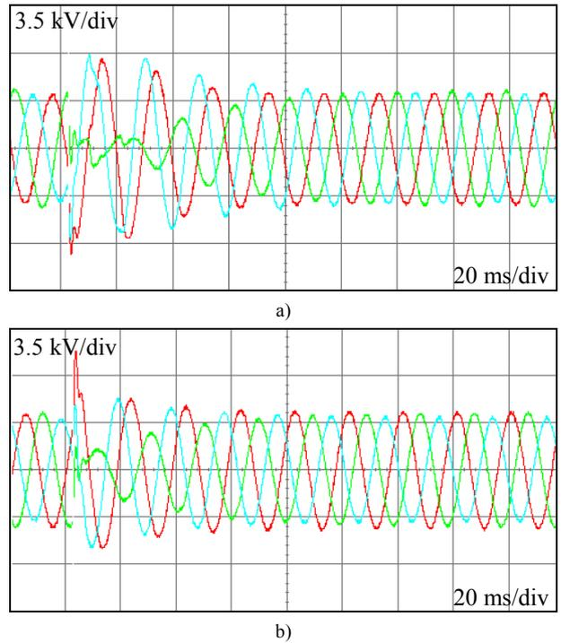
Fig. 5. Oscillograms of phase-to-ground voltages at single phase-to-ground arcing faults in the 6 kV combined grounded network (resistor + Petersen coil):
