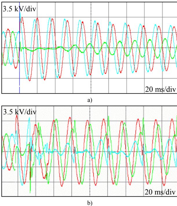
Fig. 4. Oscillograms of phase-to-ground voltages at single phase-to-ground arcing faults in the 6 kV resonant grounded network (Petersen coil, without a resistor):
