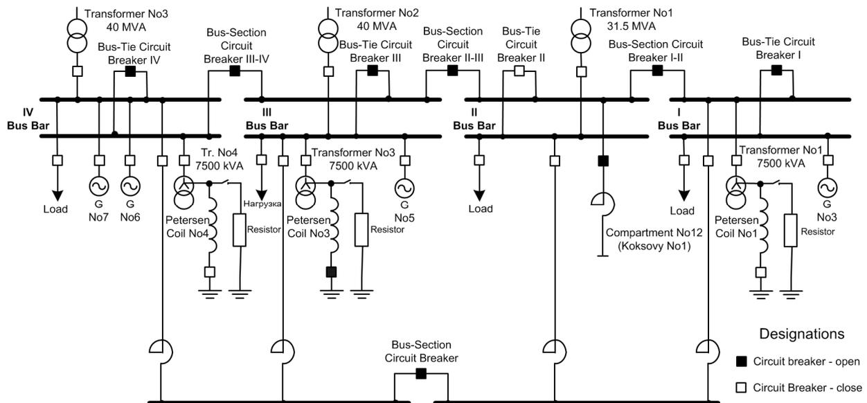
Fig. 1. Single line diagram of the Novokuznetsk Iron and Steel Plant 6 kV network where a neutral is connected to ground through a Petersen coil in parallel with a resistor.
