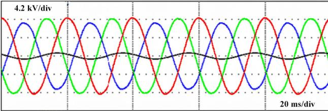
Fig. 2. Representative oscillogram recorded in the 10 kV network with neutral grounding through the Petersen coil. Blue – phase A voltage; green – phase B voltage; red – phase C voltage; black – neutral voltage.
