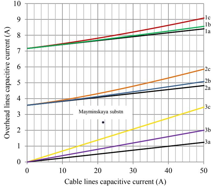
Fig. 3. Areas of proper power quality in the field of ZS voltage unbalance for 10 kV network with total capacitive current value from 0 to 60 A.
