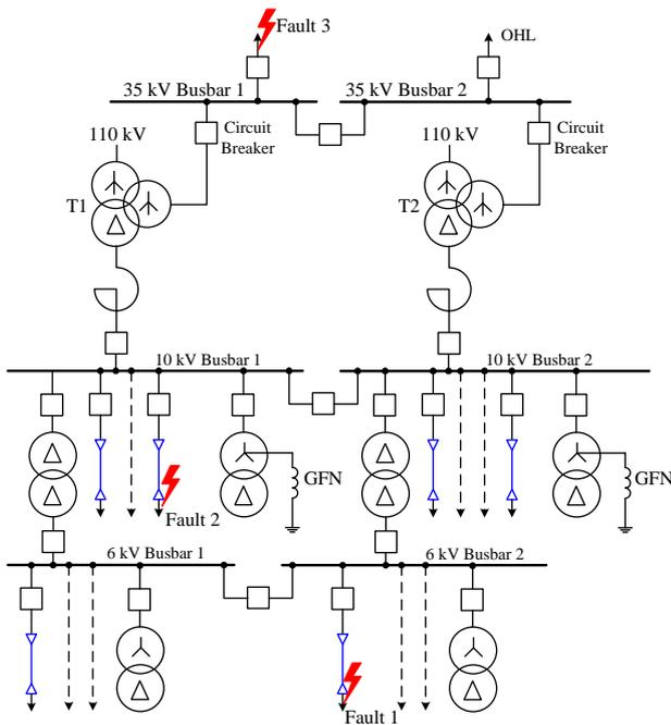
Fig. 3. Single line diagram of 110/35/10/6 kV electrical substation
