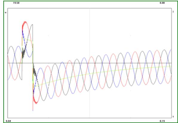
Fig. 4. Oscillogram of phase-to-ground and neutral-to-ground voltages at an arcing ground fault in 6 kV network with ungrounded neutral ( $I_{\text{fault}}=10.75 \text{ A}$ )
