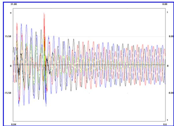
Fig. 5. Oscillogram of phase-to-ground and neutral-to-ground voltages at an arcing ground fault in 10 kV network with resonant grounded neutral through ground fault neutralizer ( $I_{\text{fault}} = 61.3 \text{ A}$ ,  $I_{\text{GFN}} = 77 \text{ A}$ , overcompensation is 25%)
