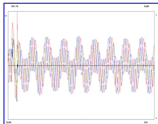
Fig. 6. Oscillogram of phase-to-ground and neutral-to-ground voltages at an arcing ground fault (Fault 3) in 35 kV network with ungrounded neutral ( $I_{\text{fault}} = 2.39 \text{ A}$ )
