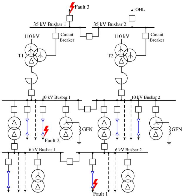
Fig. 3. Single line diagram of 110/35/10/6 kV electrical substation
