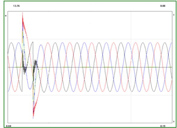
Fig. 8. Oscillogram of phase-to-ground and neutral-to-ground voltages at an arcing ground fault in 6 kV network with a neutral connected to ground through the 400-Ohm resistor
