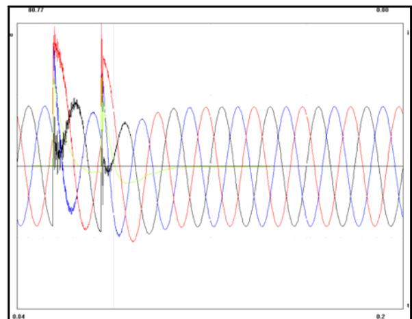
Fig. 10. Oscillogram of phase-to-ground and neutral-to-ground voltages at an arcing ground fault in 35 kV network with a neutral connected to ground through the 8000-Ohm resistor
