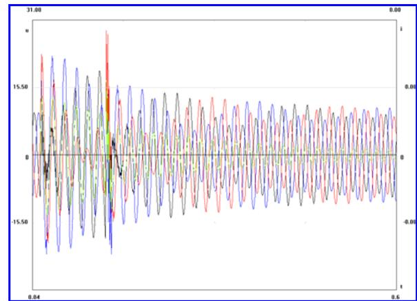
Fig. 5. Oscillogram of phase-to-ground and neutral-to-ground voltages at an arcing ground fault in 10 kV network with resonant grounded neutral through ground fault neutralizer ( $I_{\text{fault}} = 61.3 \text{ A}$ ,  $I_{\text{GFN}} = 77 \text{ A}$ , overcompensation is 25%)
